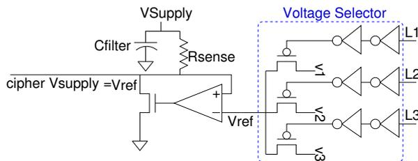
**Fig. 5.** Analog block containing the voltage selector and the suppression circuit.
