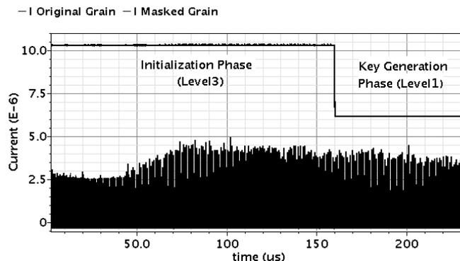
**Fig. 8.** Grain-80 with power masking blocks have smoother current pattern compared to the Grain-80 current peaks.
