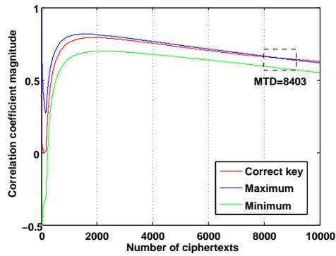
Fig. 14. Key disclosure in Grain-80 with the three alternative power levels occurs at 8k ciphertexts.
