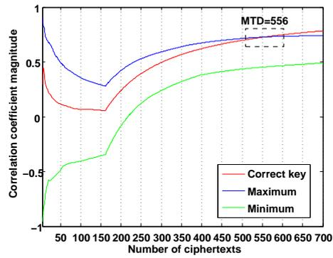
Fig. 13. Key disclosure in Grain-80 with three power levels of Table 2 occurs at 556 ciphertexts.
