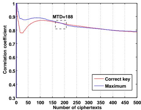
Fig. 11. Key disclosure in unprotected Grain-80 occurs at 188 ciphertexts.
