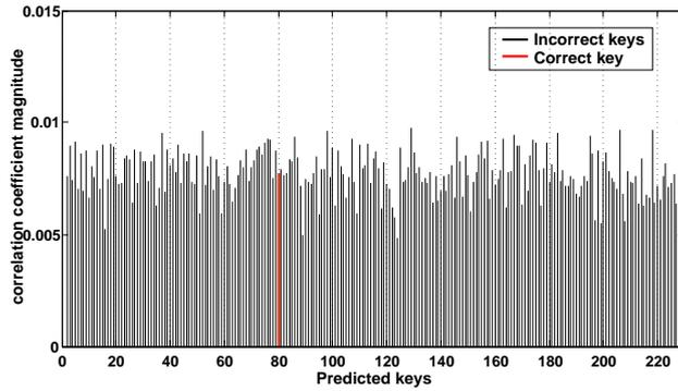
Fig. 9. Correlation coefficients of the 230 guessed keys on 3-levels protected Grain-80 after 1M encryptions.
