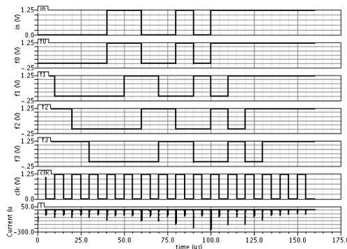
Fig. 2. The current peak is higher at times 90 $\mu$ s and 100 $\mu$ s when the sequence of state bits has a higher number of "10" or "01".
