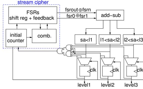
**Fig. 6.** Schematic diagram of the digital modules added to the original cipher.
