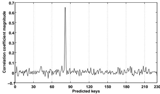
Fig. 10. Correlation coefficients of the 230 guessed keys on unprotected Grain-80 after 5k encryptions.
