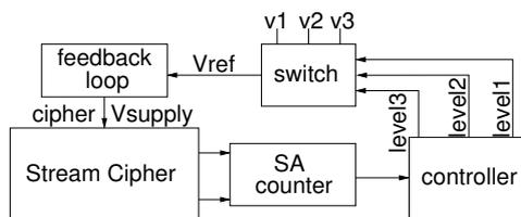
**Fig. 4.** Schematic diagram of the suggested countermeasure.
