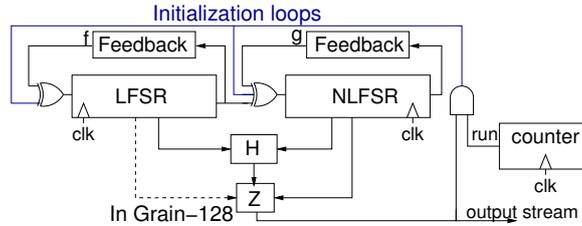
**Fig. 7.** Schematic structure of the Grain cipher.
