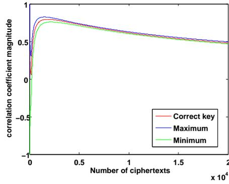
Fig. 12. Key disclosure in Grain-80 with two power levels can occur for ciphertexts larger than 20k.
